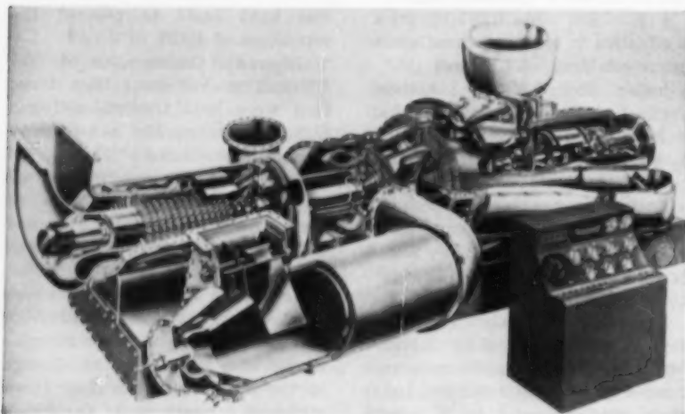
Cut-away view of the Clark Mark TA gas turbine
